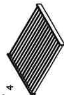
4 Cooking Grates (2) (Installed with the closed end of the channels facing up and resting flat on top of the Radiant Glass Panel with no space between the grid and the glass.)
